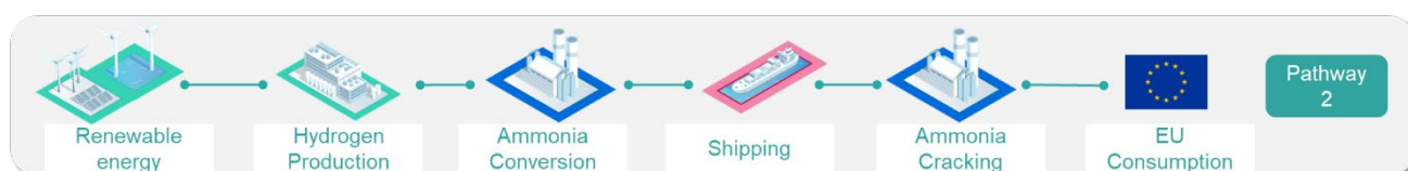
Figure 15 – Schematic of ammonia shipping transport pathway
